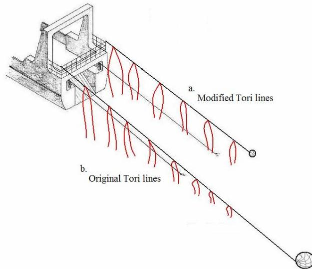
**Figure 2.** BSL (tori lines) designs under trawlers licence conditions in the Falkland Islands. a) Modified tori lines design implemented by FIFD 2009, b) Original tori lines design implemented by FIFD 2004-2008.
